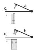
The axis of the hinge should be x mm above the top edge of the safety switch and in the same plane. a = Actuating radius to the plane of the actuator b = Actuating radius in line with the plane of the actuator x = Axial misalignment
