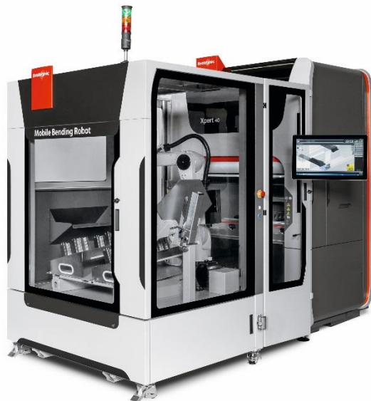
[03] A "mobile bending cell" makes conventional press brakes fit for automation
