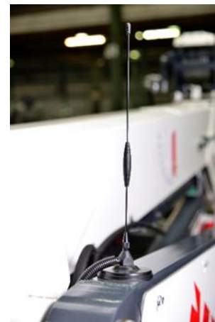
An antenna receives the signals from the wireless switches and sensors and passes them on.
