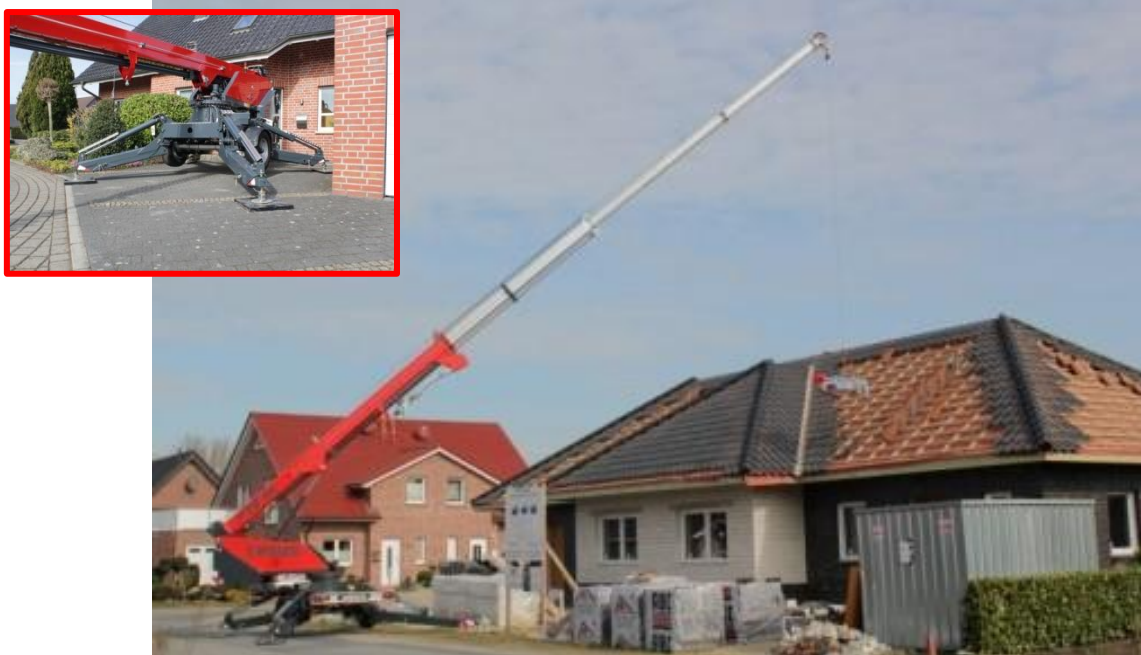
The "Sky Worker PTK 25" aluminium crane was developed for work in confined spaces.
