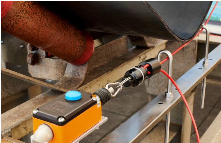
The new belt-rip detection system detects any rip in a conveyor belt early on, minimising subsequent damage
