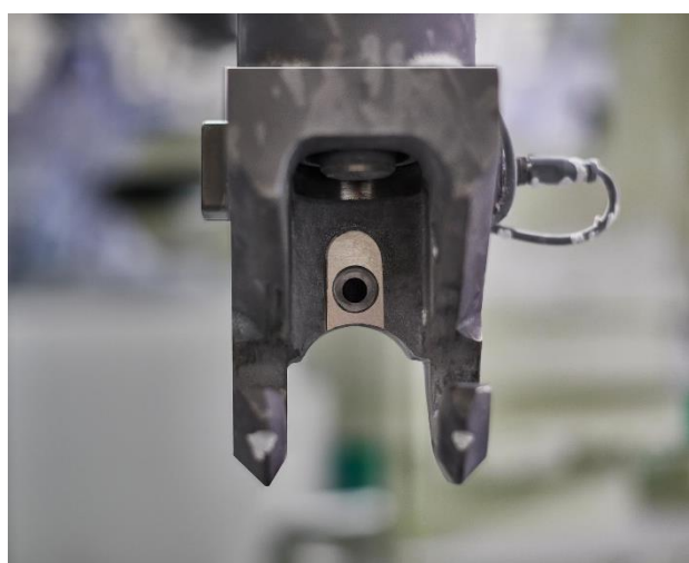
The robot gripper (a) with a retrofitted wireless sensor central to the bolt receptacle (b)
