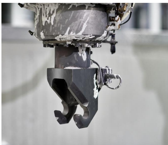
The robot gripper (a) with a retrofitted wireless sensor central to the bolt receptacle (b)
